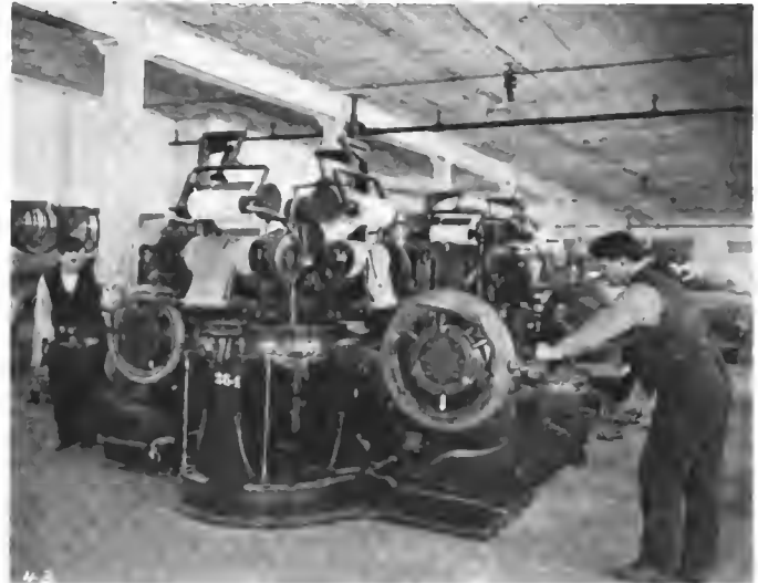
Machine Rolling Fabric Down After It is Stretched
